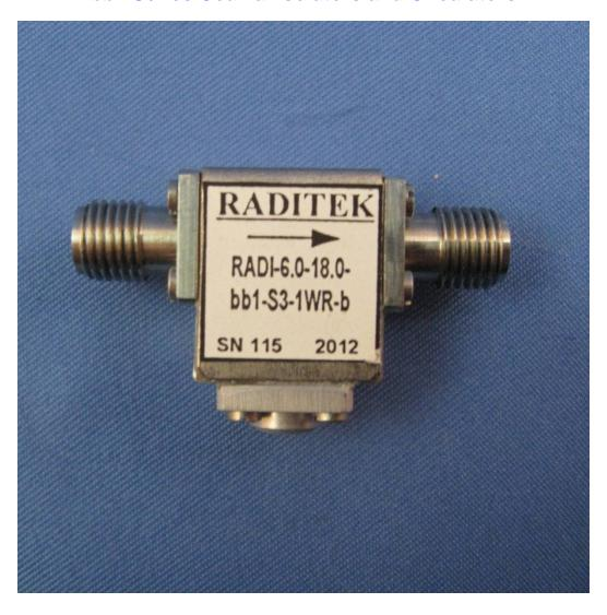
RADITEK'S Our bb1 Series of Coaxial Isolators and Circulators operates from 5.8-31 GHz at 10% Bandwidth Standard or up to 20% option. 1-2 Watts Reverse power and 10 Watts Forward power. Connector options include SMA, 3.5 and 2.9(K). Dimensions: mm (In), (W) 0.5(12.7) x (L) 0.6(15.3) x (H) 0.41(10.5).
